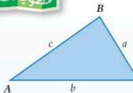
$$k = \frac{1}{2} ab \sin C \quad k = \frac{1}{2} ac \sin B \quad k = \frac{1}{2} bc \sin A \quad \text{الرموز:}$$
